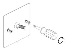
\* Please ensure screws are sufficiently tight to support the product but please do not over tighten as this may cause some deformation to the plate or damage the
