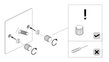
\*\* Do NOT use a standard screw driver to tighten the coin caps. This may damage the cap and is not covered under warranty. Plastic coin cap tool
